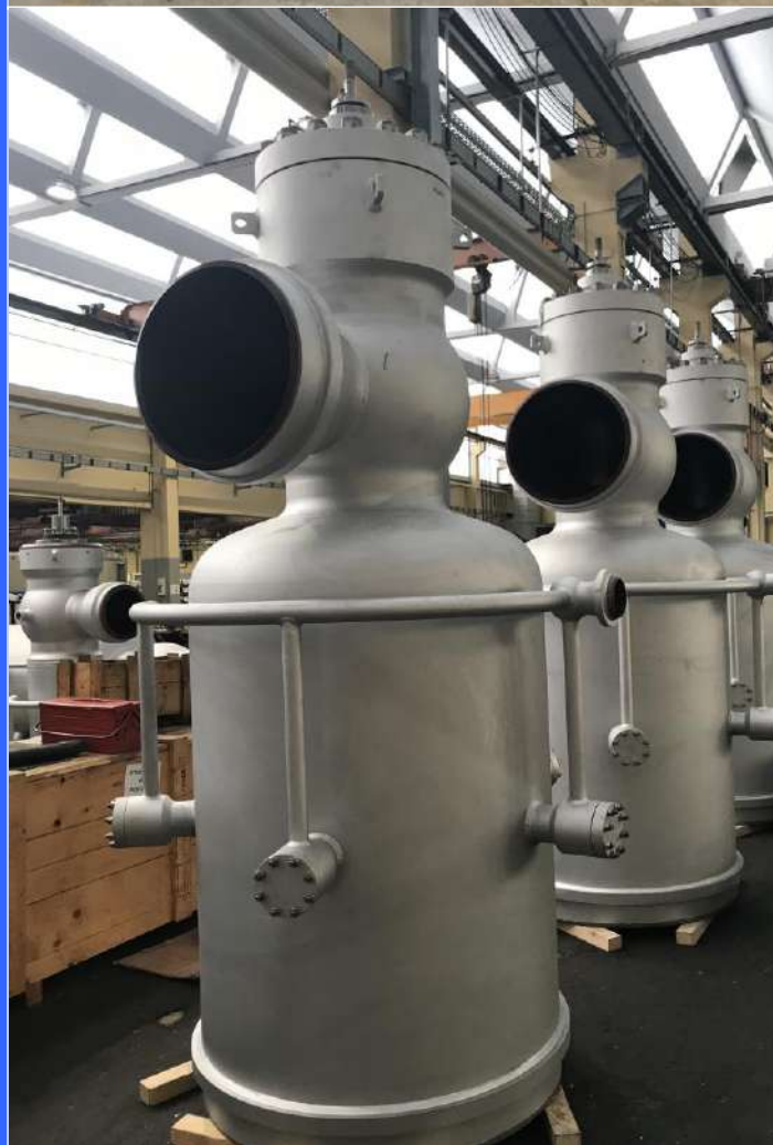
Corpi valvola by pass turbina di materiale: grado 91 - 22 - 11 By-pass turbine control valve body material: gr. 91 gr. 22 gr. 11
